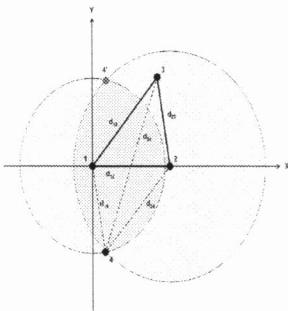
**Fig. 3:** Trilateration. Sensor 1 is at the center of coordinate system. Sensor 2 on the positive x-axis and Sensor 3 in quadrant one or two. The coordinates for the fourth sensor are calculated with  $d_{14}$  and  $d_{24}$ . One of the two intersections of the circles is the location of Sensor 4. A comparison of the measured distance  $d_{34}$  to the estimated distance reveals the final location.
